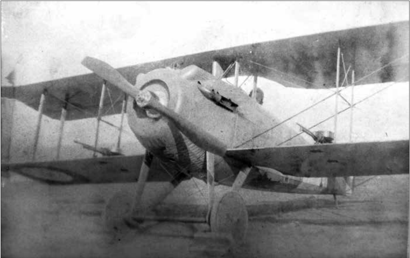
SPAD S.VII, SFA S.1083, after Costes had installed two Lewis guns on the lower wings. In addition, the exhaust pipes had been cut away and shortened. The early 'winter' cowling cannot have helped the engine cooling in the heat of a Macedonian summer. : David Méchin
