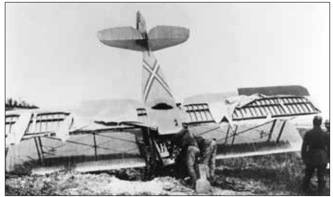
Above: Another SPAD which came to grief owing to fabric stripping off the top wing.
