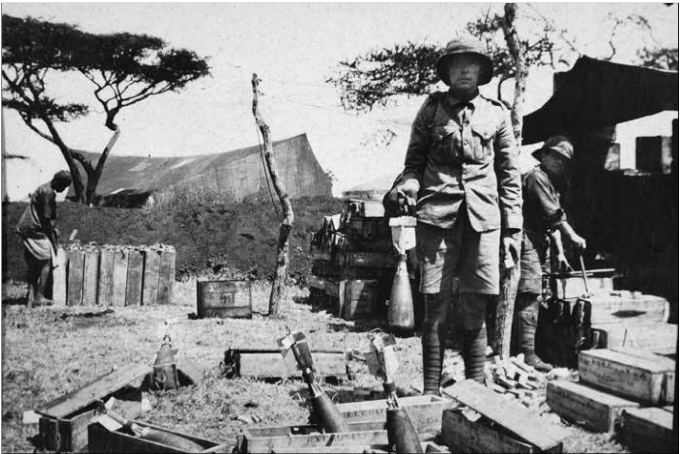
The Armoury at Mbuyuni. Bell mentions that the bombs used in East Africa did not explode at first - only the primer went off; not the main charge. On examination it was discovered that the T.N.T had liquified and soaked into the primers. Thereafter the primers were stowed apart and only inserted just before the bombs were loaded on to the aircraft. :both Ray Vann/Mike O'Connor Collection
