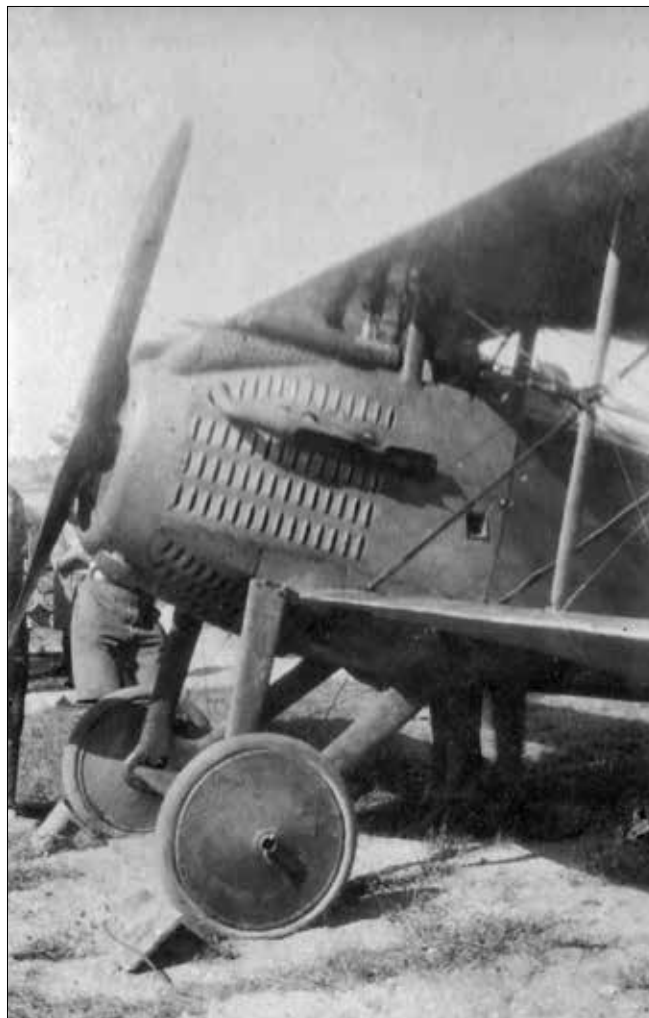
SPAD VII S.1073 gifted by the French to the RFC in June 1917. This view shows the second Vickers gun fitted. In addition to this, and various other modifications, the exhaust pipes have been cut away in the same manner as on S.1083, the first SPAD used by Costes. S.1073 was delivered to the RFC on 5 June 1917 as a reciprocal gesture after the RFC had given the French a BE12 back in January 1917. This SPAD went to 17 Squadron on 25 June but was not used operationally until 12 July. :CCI Archive
